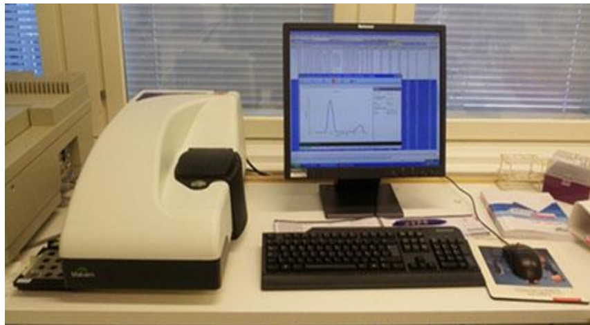
Figure.2 Photography representation of Malvern zetasizer used for finding particle size analysis
