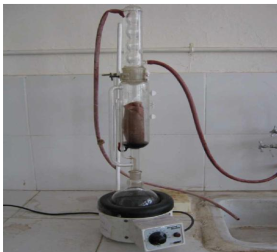
Figure.1 Soxhlet apparatus for the extraction of different plant Extracts
