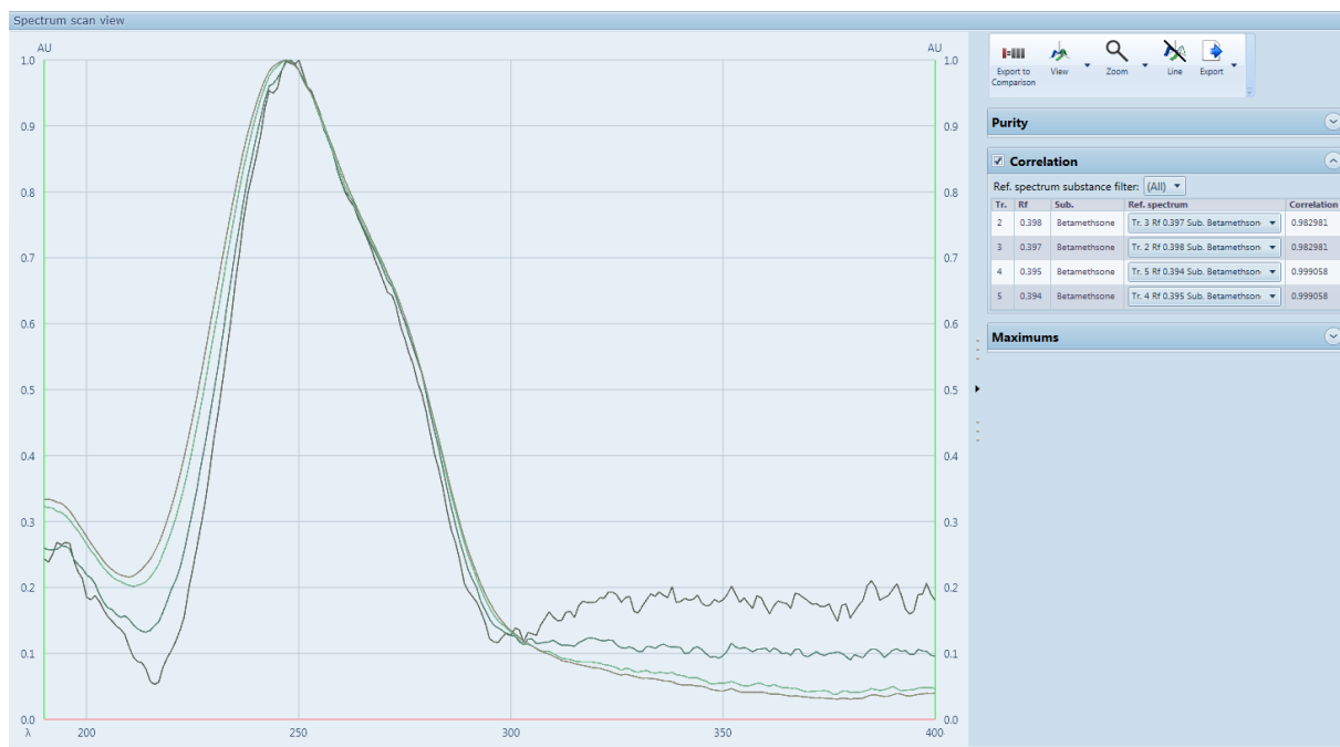
Fig. 2: The overlain UV spectra of 1000 µg/ml Betamethasone valerate (API and sample) between 200 and 400 nm
