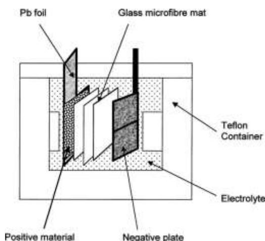
Figure 5 shows the schematic representation of cell used in electrochemical experiments
