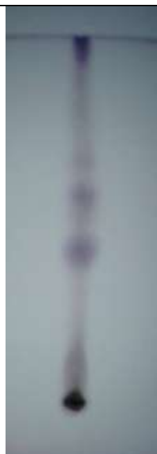
Figure 8: TLC shown pattern of steroid and triterpenoid after spraying with anisaldehyde -H 2 SO 4 of ethanolic extract
